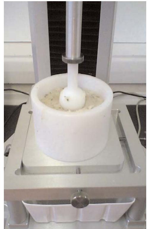
Penetration of prepared sample in duplicate.
