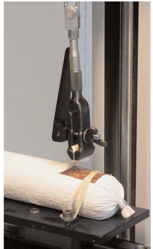
Test assembly configured with assisted peel table to maintain 90° throughout analysis.
