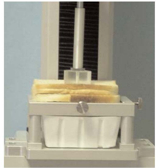
Two slices are presented to the test probe and deformed to 50%.
